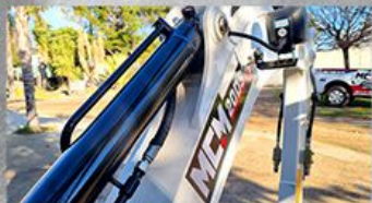
Protected Hydraulic Hoses
