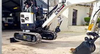
Variable Chassis Width
