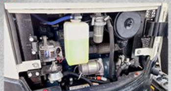
3-Cylinder Kubota Engine
