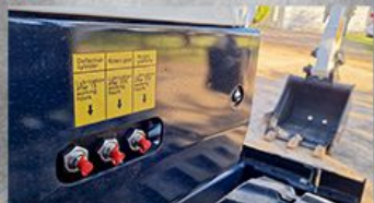
Centralized Grease Bank
