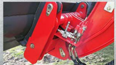
Hydraulic Quick Hitch
