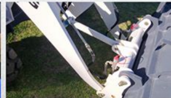
Hydraulic Quick Hitch
