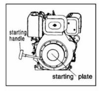
D.In cold weather, when your engine is hard to start, remove the rubber plug of the cylinder head cover and add 2ml of lube oil before starting.
